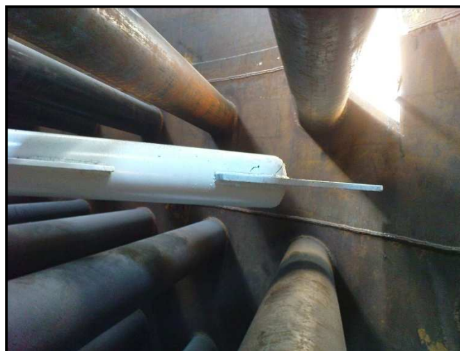
Figure 6. A view of an FF stirrer inside a crystalliser.
